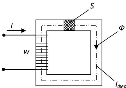
$$a) R_M = I_{\phi}/\mu_a S \quad b) R_M = S/I_{\phi} \quad c) R_M = S I_{\phi}/\mu_0 \quad d) R_M = I_{\phi}/\mu_0 S$$
