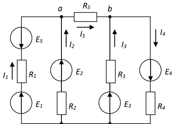
a)  $I_2R_2 + I_3R_3 + I_5R_5 = E_2 + E_3$
